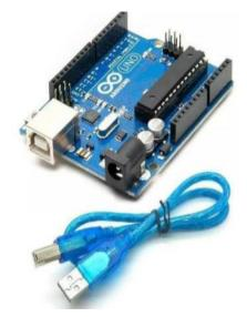
Fig. 7: Microcontroller Arduino UNO
